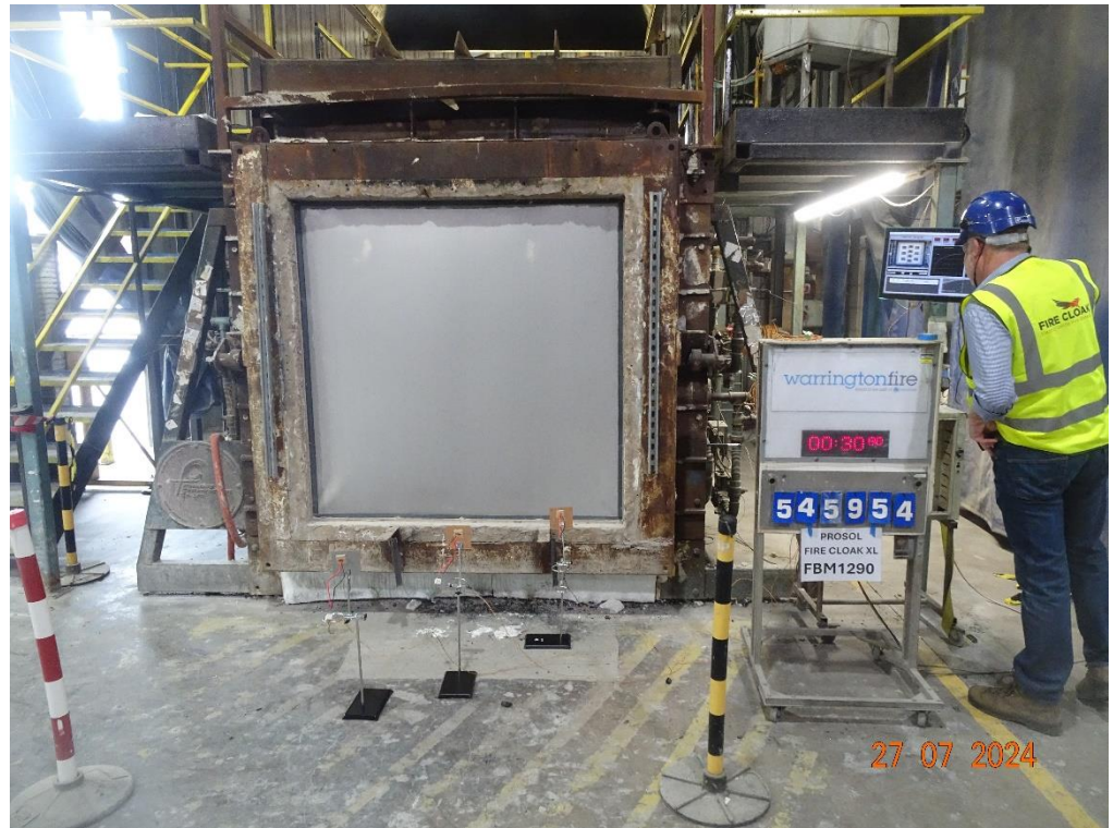
The unexposed face of the test assembly after 30 minutes of testing
