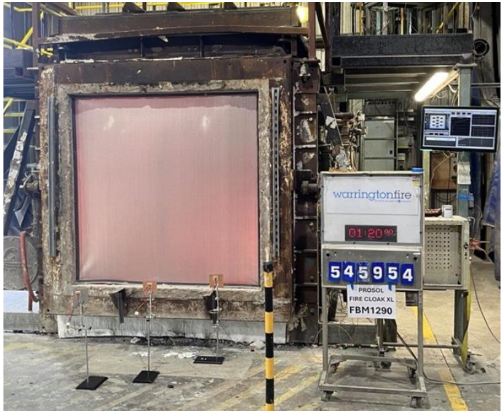
The unexposed face of the test assembly after 80 minutes of testing
