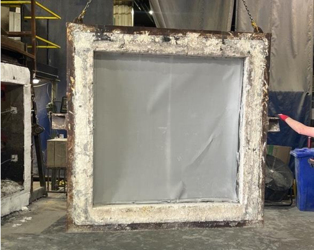
The exposed face of the test assembly after the end of the test
