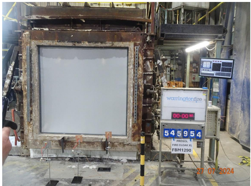
The unexposed face of the test assembly before the start of the test
