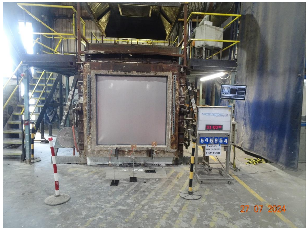
The unexposed face of the test assembly after 60 minutes of testing
