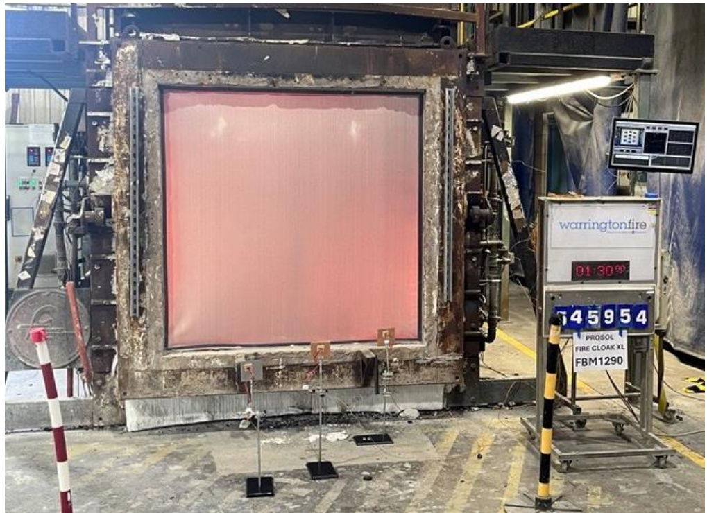
The unexposed face of the test assembly after 90 minutes of testing
