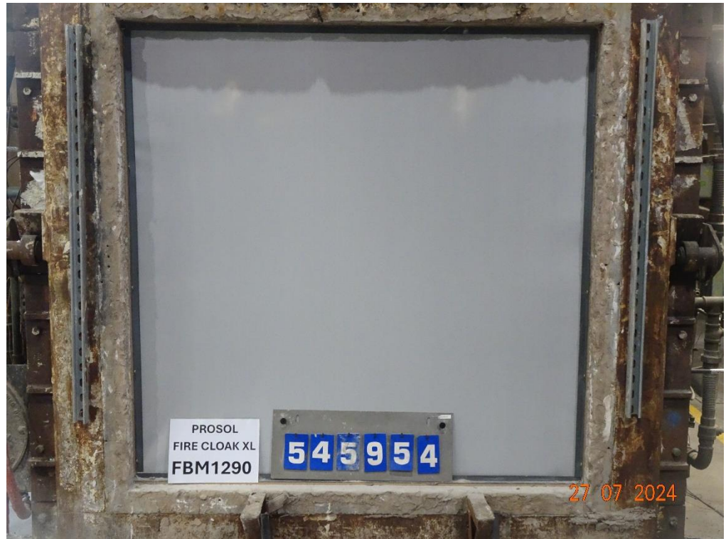
The exposed face of the test assembly before the start of the test
