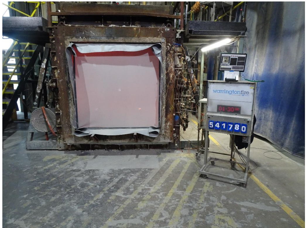
The unexposed face of the test assembly after a test duration of 90 minutes
