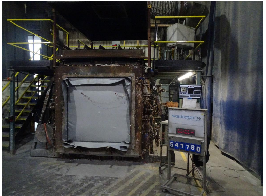
The unexposed face of the test assembly after a test duration of 20 minutes
